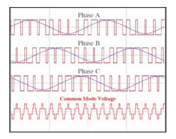
Figure 2: PWM two-level voltages principle
