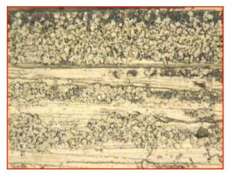
Figure 6: Craters on a roller surface (x930)
