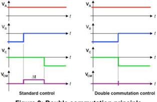
Figure 9: Double commutation principle
