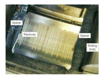
Figure 7: "Washboard" pattern of a raceway
