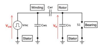
Figure 4: Equivalent low-frequency CM circuit
