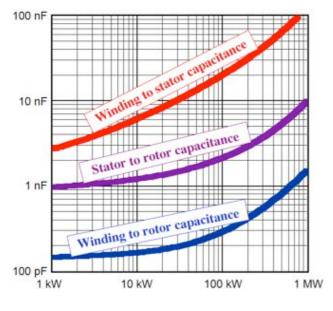
Figure 3: Motor capacitances vs. power
